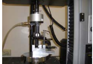
Figure 1. Shear Bond Test Set-Up Without Sample
