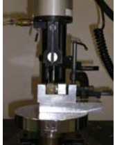
Figure 2. Shear Bond Test Set-Up During Test
